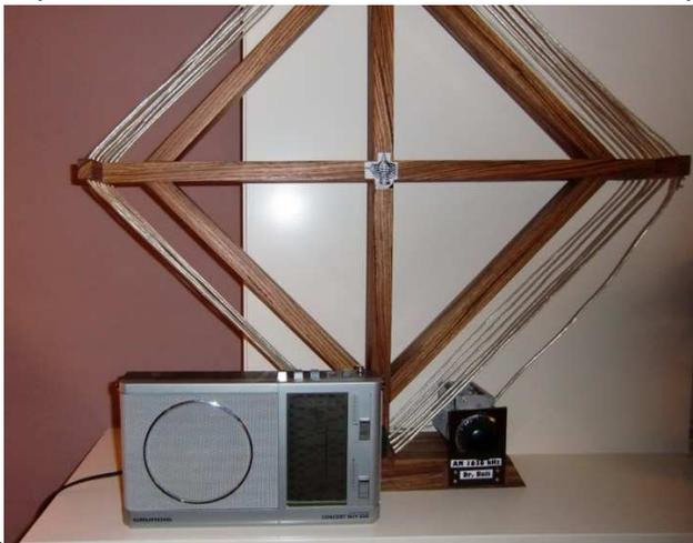
loop. picture 2 MW loop on a wooden frame.
